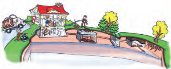
Typical on-site wastewater treatment system
